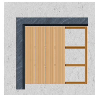
Basic installation substructure; 300mm on center maximum joists. (250mm on center for commercial applications)
